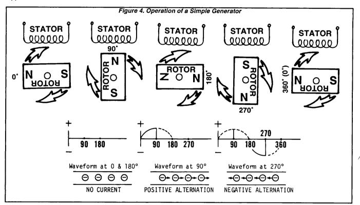
With alternating current (AC), the electrons flow first in one direction, then reverse and move in the opposite direction. They will repeat this cycle at regular intervals. A wave diagram, called a "sine wave" shows that current goes from zero to maximum positive value, then reverses and goes from zero to maximum negative value. Two reversals of current flow is called a cycle. The number of cycles per second is called frequency and is usually stated in "Hertz".
